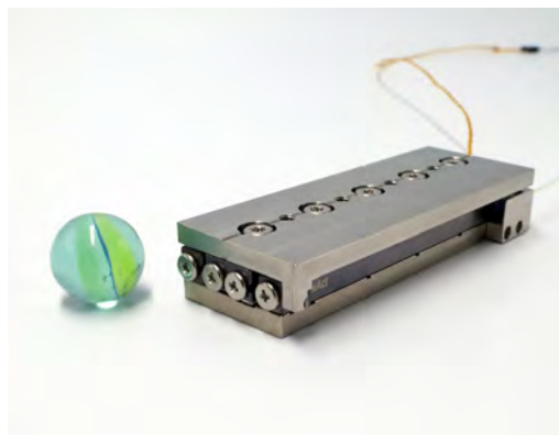
SLC-2475-F stage for highest positioning accuracy under cryogenic conditions.
