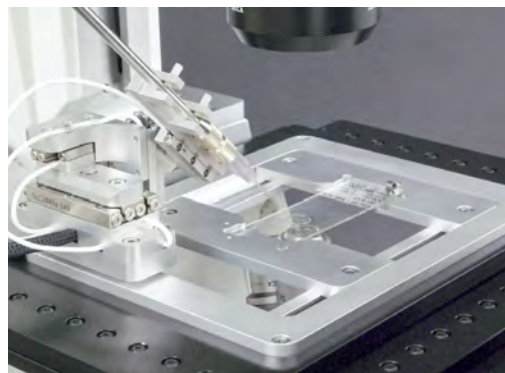
A customized four-axis micro-manipulator allows positioning of tools with nanometer precision in front of the objective lens.
