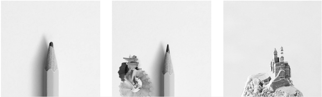
A tiny castle printed on the tip of a sharpened pencil by using a high precision microscope stage for two-photon polymerization.
