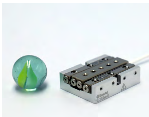
SLC-1730 with U-shaped base (option -W) for higher mechanical strength, which is highly recommended for non-magnetic stages, UHV stages that are baked out and stages that are subject to torques.
