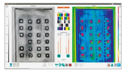
T-SENSE FMI Grafic user interface with different filters side by side. All parameters are intuitively customizable. There is also an image overlay technique of the visual and the THz image
