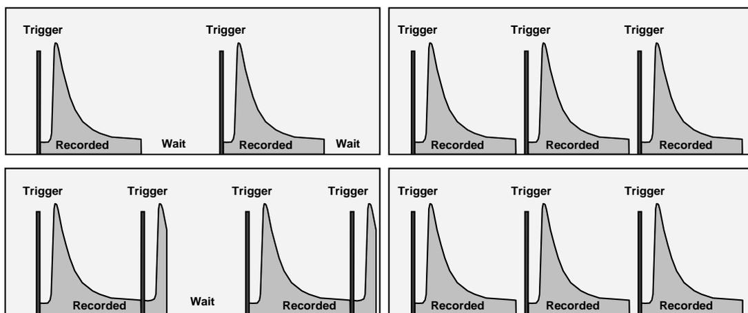
Recording sequence with waiting for trigger (left) and optimised sequence (right)
